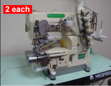
Megasew MJ2600SD-356 3 NDL, Cover Stitch, Full Auto Left Side Trim, Waste Removal $1,995.00 each
