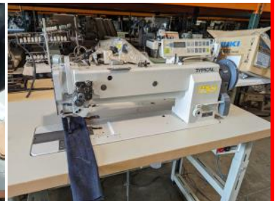
Typical GC-20606-1L18 SN, Walking Foot, Auto 18" Long Arm, Electric/Air $3,500.00
